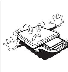
By adjusting 4 corners of the scale, set the scale even using the built in scale leveling indicator.
