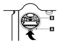
So that weighings can be carried out below the working surface (below-the-balance weighing), your balance is provided with a special hanger.
