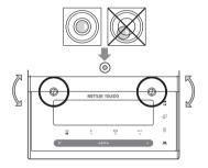
The balance has a level indicator and two adjustable leveling feet to compensate for slight irregularities in the surface of the weighing bench. The balance is exactly horizontal when the air bubble is in the middle of the level glass.
