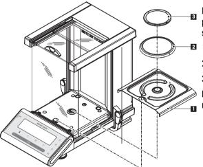
Push the side glass doors back as far as will go and place the following components on the balance in the specified order:
