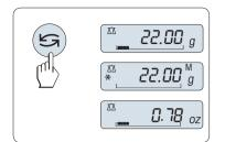
The « key can be used at any time to toggle between weight unit "UNIT 1", "RECALL" value (if selected) and weight unit "UNIT 2" (if different from weight unit 1) and the application unit (if any).
