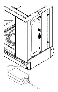
Connect the AC adapter to the connection socket on the back of the balance (see figure) and to the power line. Secure the connection to the balance by screwing the plug tight.
