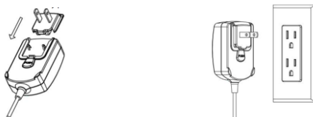
Figure 2-4. Connecting the AC adapter to AC supply
