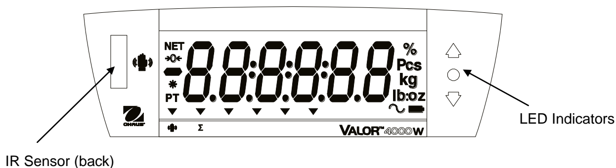
Figure 1-2. Valor 4000 Back Display.
