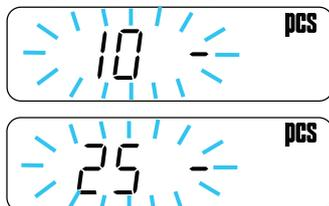
When sample weight is light and the counting error could become large, the balance will request you to use larger number of samples. Place the displayed number of samples on the pan and press the **PRINT** key to store the unit weight.
