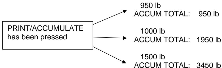
Once a successful accumulation has occurred, press the LOCAL/TOTAL button to toggle the display through the current local weight, current total weight, accumulated total, and the number of accumulations that make up the total.
