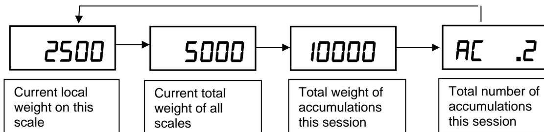
Note: If the system is not setup correctly, the "error" icon and message "Err" will be displayed when trying to view the total weight. See section titled "Totalizing Setup".
