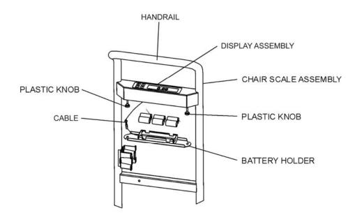
Figure 4. Replacing Batteries
