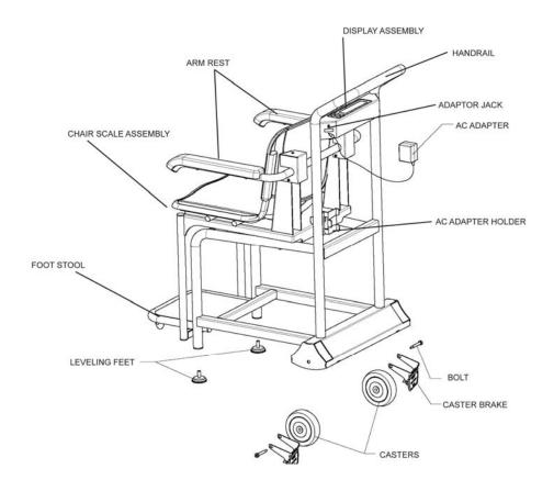
Figure 2. Assembly of the 2595KL
