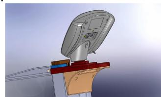
Place the display module on top of the pillar and use the Phillips screw to fasten the module to the pillar
