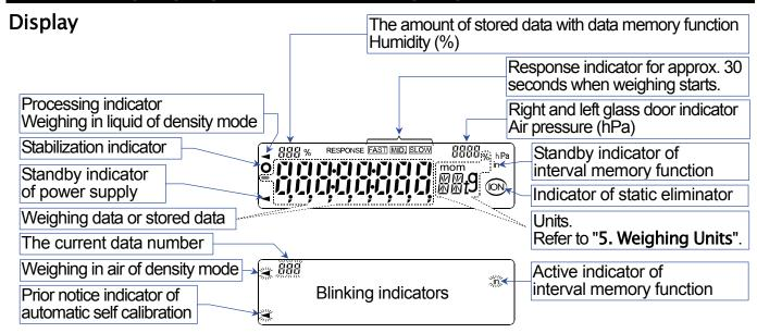
The interval memory function is used to store periodical weighing data. Refer to "12. Data Memory".
