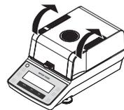
2 Carefully remove the sample handler from the sample chamber.
