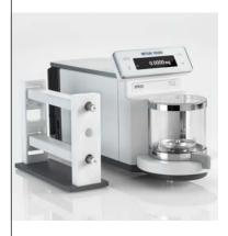
To help to address one of the major challenges in micro-weighing, the freestanding ionizer removes electrostatic charges on samples and containers.
