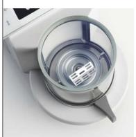
This flexible holder is perfect for ensuring that tubular shaped samples can be placed securely on the balance (e.g. stents).
