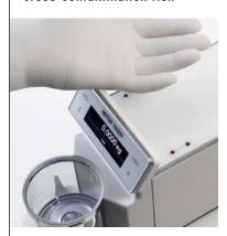
SmartSens infrared sensors enable you to operate the draft shield doors with the wave of a hand. This touch-free balance operation reduces the risk of crosscontamination.
