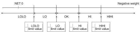
Note: To start take-away check weighing, be sure to use the TARE key to tare the weight of the container filled with objects. The ZERO key may zero the display, but the scale goes below the zero point by taking away the objects. Then, the auto-tare function or TARE key does not work.
