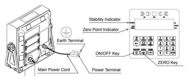
$\triangle$ Please confirm that the local voltage and the receptacle type are correct for your scale.
