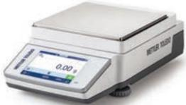
A white precision balance with a flat weighing pan and a digital display showing 0.00. The brand name 'METTLER TOLEDO' is visible on the front.    | Readability: <b>10 mg / 100 mg</b> <ul style="list-style-type: none"><li>• MR1002</li><li>• MR2002</li><li>• MR3002</li><li>• MR4002</li><li>• MR6002</li><li>• MR6001</li></ul> |
